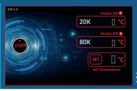
uP controlled heater module with 5" touch screen allows to control set temperatures and visualize 20K and 80K temperatures.
