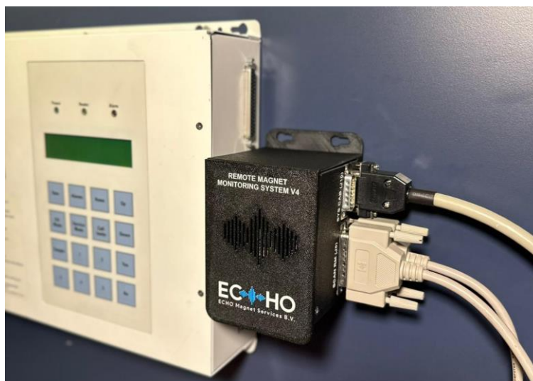
Illustration 3.5 Example photograph showing the finalized mechanical assembly, with the RMMS V4 securely mounted and interconnected with the Magnet Monitor.
