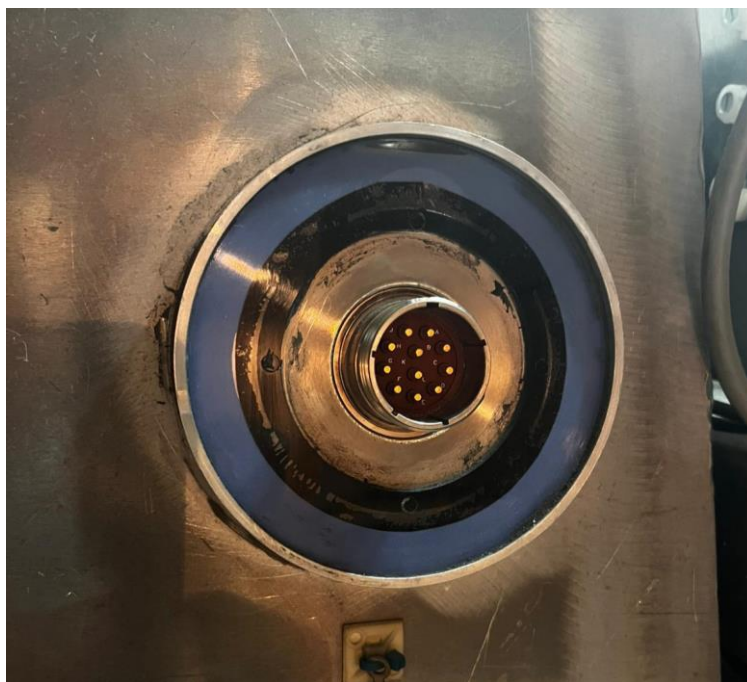
Illustration 4-3: 11-pin Deutsch connector port on Philips Magnet Turret
