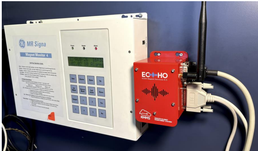
Illustration 3.5 Example photograph showing the finalized mechanical assembly, with the RMMS V4 securely mounted and interconnected with the Magnet Monitor.
