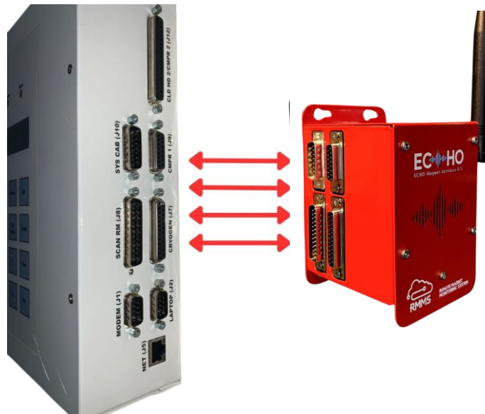
Illustration 3.3 Side-by-side view of the Magnet Monitor (right side) and the RMMS V4 (left side)
